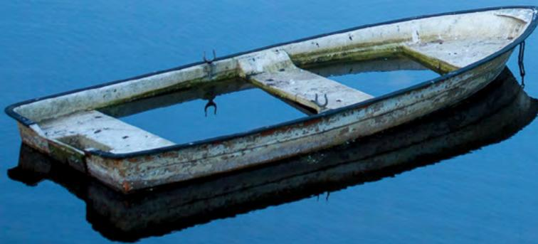
Vessels with level flotation have buoyancy installed to national standards high up in the extremities, allowing the vessel to float level with the waterline if it becomes swamped or flooded. Whether the vessel capsizes or stays upright, level flotation offers a number of advantages for people who find themselves in this predicament.
