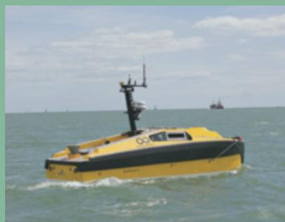
SeaWorker USV autonomous surface vessel conducting surveillance of the ocean floor – Ocean Infinity
