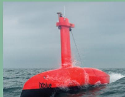
DriX USV Remotely operated vehicle using autonomous docking underwater technology – iXblue and Forssea
